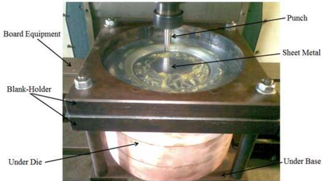
Fig. 7. Components used for the incremental sheet forming.
